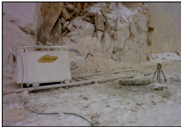
Figure 1. Diamond wire cutting machine performing in marble quarry.
